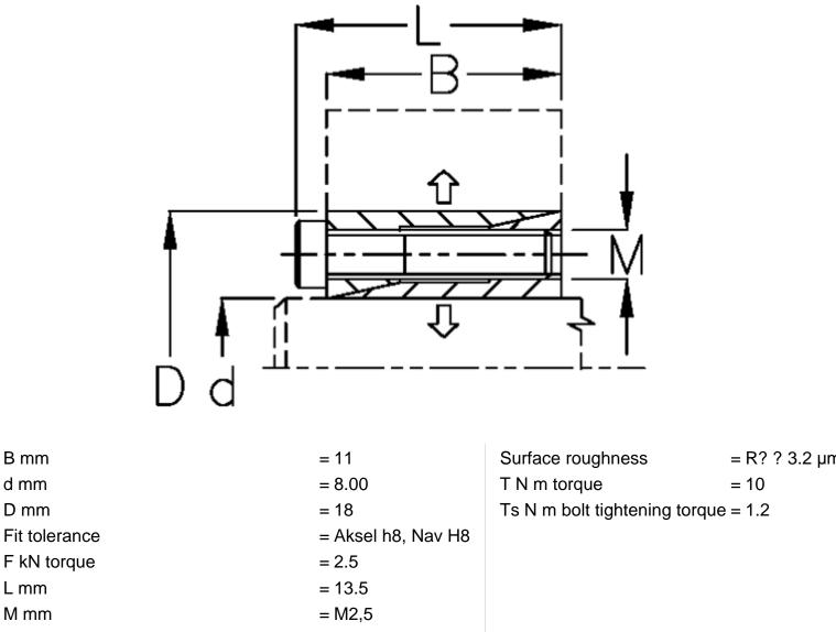
P N/mm2 surface pressure on shaft/hub = 50
